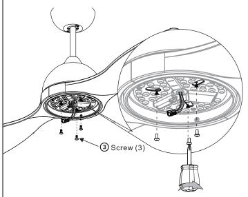
4 Plug the male connector into female connector from LED Light.
