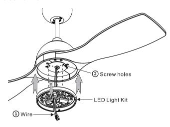
③ Attach LED Light Kit to the fan assembly by tightening screws (3).
