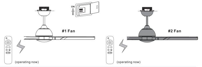
**NOTE:** For more than two fans, the same rules apply. Make sure only one fan at a time is connected to power when doing the Remote Setting. Already completed fans should be disconnected until all fans have completed the Remote Setting process.
