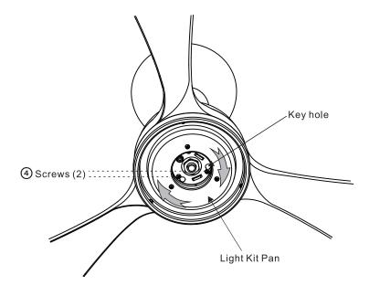
(5) Attach screw (removed from step (1)), and tighten 3 screws.
