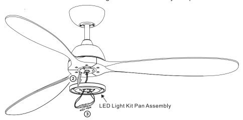
4 Rotate the Light Kit Pan slightly until two pre-installed screw heads are engaged in the narrow end of key holes.
