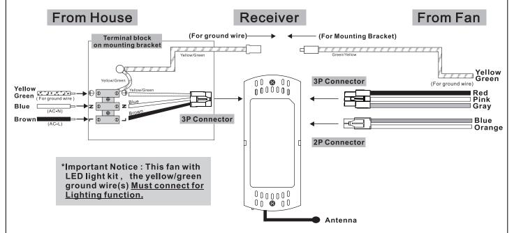
"Special note: All Yellow/green grounding wires, from <u>Fan Assembly / Mounting bracket</u>, must be well attached to House Ground/Earth to prevent flickering of LED."
