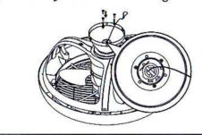
[Step 4] Please use safety steel wire to fasten the hook indeed. This will allow hands free wiring.
