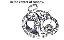
[Step 3] Install 3 mount screws and tighten securely.
