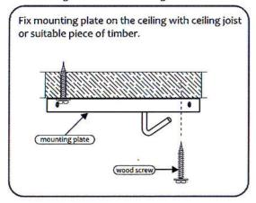
Installing in the wall ceiling/ Installing in the Cement ceiling:
