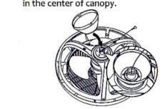
[Step 3] Install 3 mount screws and tighten securely.
