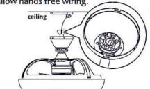
[Step 8] Lift fan to mounting plate, aligning the "L" shape holes with the screws on the mounting plate. Turn the fan anti-clockwise to lock in position. Install the other two screws and tighten securely.
