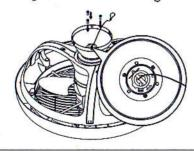
[Step 4] Please use safety steel wire to fasten the hook indeed. This will allow hands free wiring.
