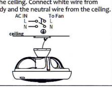
[Step 6] Lift fan to mounting plate, aligning the "L" shape holes with the screws on the mounting plate. Turn the fan anti-clockwise to lock in position. Install the other two screws and tighten securely.
