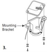
Install mounting bracket to Outlet box in ceiling using washers and the mounting screws provided with the outlet box.
