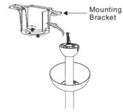
Lift fan assembly onto mounting bracket.
