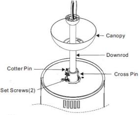
(2)Insert the cross pin through yoke & downrod and secure with cotter pin.
