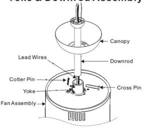
(1) Feed motor lead wires through canopy and downrod and insert downrod into yoke.
