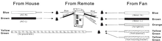
Secure with twist - lock wire nuts (Included).
