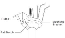
Carefully lift fan assembly onto mounting bracket. Rotate fan so that the notch on the ball engages the ridge in the mounting bracket.
