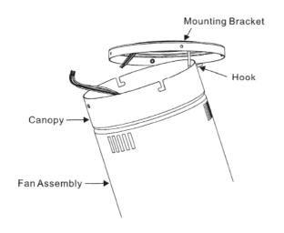
Lift the fan assembly and hang onto the hook on mounting bracket. This will permit you to make the electrical connections without having to hold the fan up as well.
