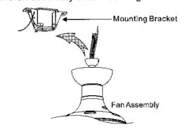
Rotate fan so that the groove on the ball engages the ridge in the mounting bracket.
