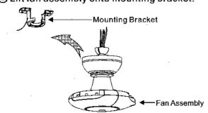
② Rotate fan so that the groove on the ball engages the ridge in the mounting bracket.
