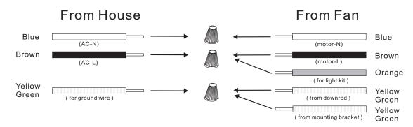
Secure with twist - lock wire nuts (Included).
