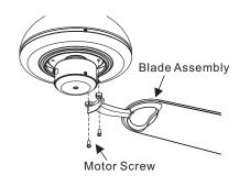
Mount blade assembly to motor housing by motor screws provided.
