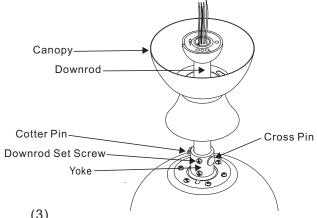
Insert the cross pin through yoke & downrod and secure with cotter pin.
