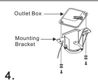
Install mounting bracket to Outlet box in ceiling using washers and the mounting screws provided with the outlet box.
