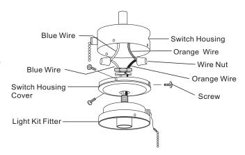
Attach switch housing cover and light kit assembly to switch housing by 3 original screws.
